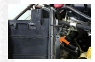
» Install the battery cover by lining up all the clips with the base and firmly pushing it into position.
