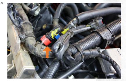
» Once the collars have been removed, have some rags ready, and gently pull up on the connection and move aside.
