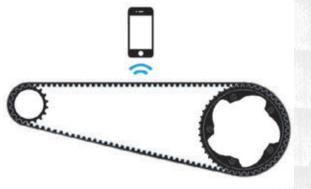
From the App, click the Tension icon and then click Measure From the App, click the Tension izon and then click Measure. Heldő the device microphone (les sure microphone is 'on') facing the bell. Plock the belt so that it vibrates similar to a guitar string. Rotate the crank ik furn and repeat the frequency measurement. Compare your belt's frequency to the chart op 44 to review any necessary tension adjustments. The Gates Carbon Drive Mobile App works best in a quiet environment.
